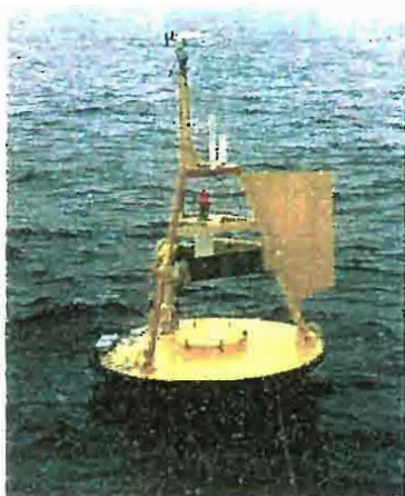
Figure 1. Station 42036 (28.51 N 84.51W) which is owned and maintained by National Data Buoy Center (NDBC). Site elevation: sea level; Air temp height: 4 m above site elevation; Anemometer height: 5 m above site elevation; Barometer elevation: sea level; Sea temp depth: 0.6 m below site elevation; Water depth: 53.0 m; Watch circle radius: 126 yards.
